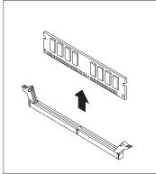
Figure 11. Removing the memory module
